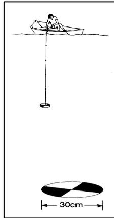
**FIGURE 3:** THE USE OF A SECCHI DISC TO ASSESS VERTICAL WATER CLARITY. The Secchi disc is lowered into the water until the black and white quarters are no longer distinguishable. The length of the rope from surveyor to the disc is then recorded.
